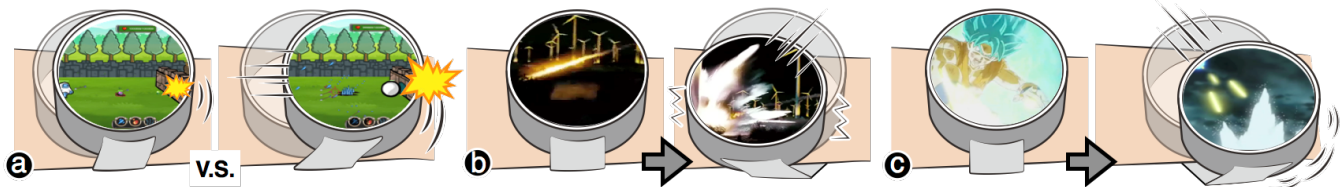
Figure 1. Jetto creates lateral displacements on a smartwatch to simulate force impacts caused by a virtual object pushing or colliding into the edge of the watch screen, creating an illusion that the impact is created by a real object colliding inside the smartwatch. It simulates forces in different (a) magnitudes (e.g., weak vs strong); (b) directions; and (c) locations and durations.
